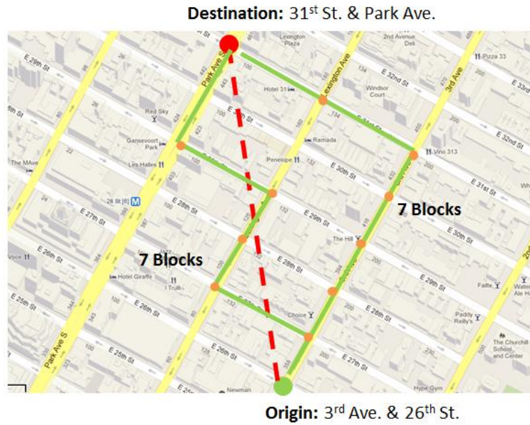
Figure 12: With the Manhattan Heuristic, the agent knows the destination coordinates, but not obstacles in its way and determines its distance in horizontal and vertical spaces like city blocks.
