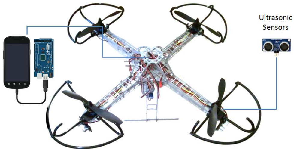
Figure 2: Fully constructed frame, calling out location for phone and controller housing, with ultrasonic sensor positions.
