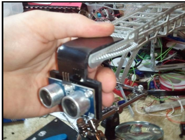
Figure 5: Custom mounts for ultrasonic sensors.
