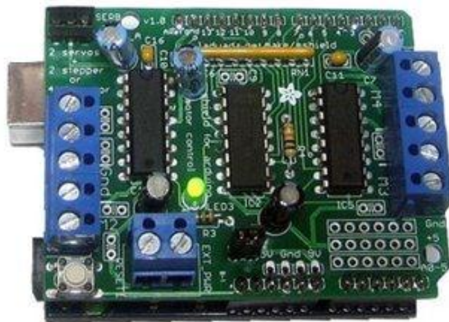
Figure 9. Adafruit Motor Shield Sitting on Arduino Microcontroller
